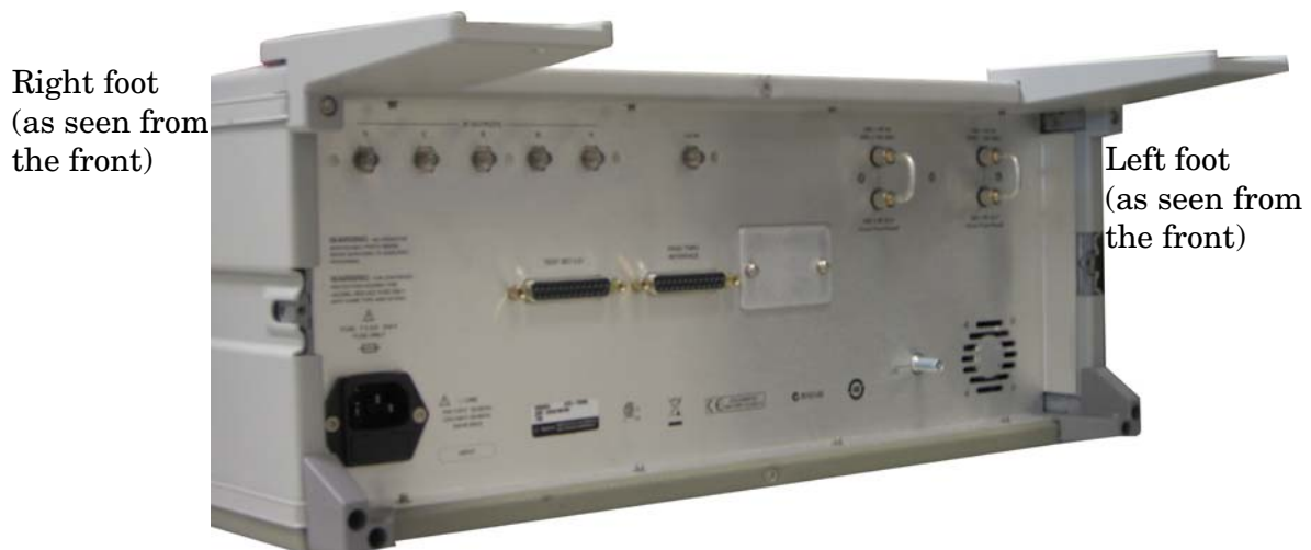
Figure 9 Install Locking Feet on N5261/62A
